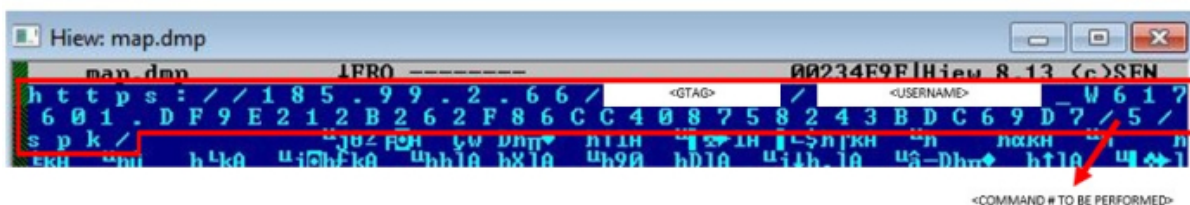
Figure 7: The memory dump of TrickBot “map.exe” showing the first request to its C&C
