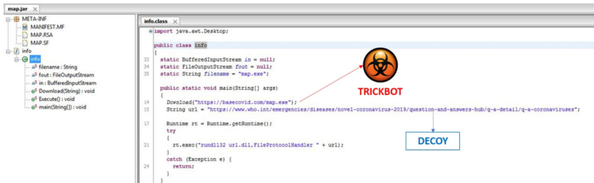
Figure 4: The second stage downloader “map.jar” will download and execute the main malware “map.exe”
