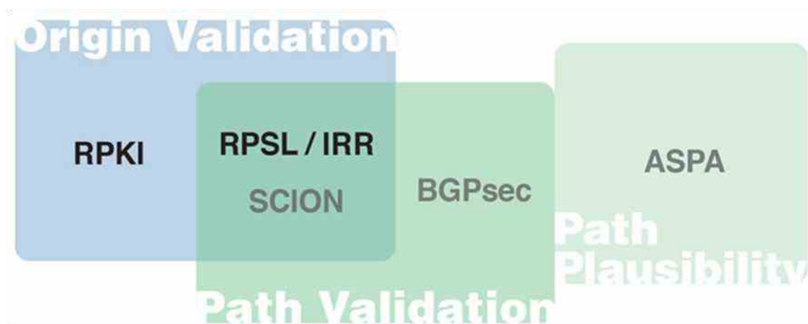
Figure 5. Mapping of current routing security techniques
