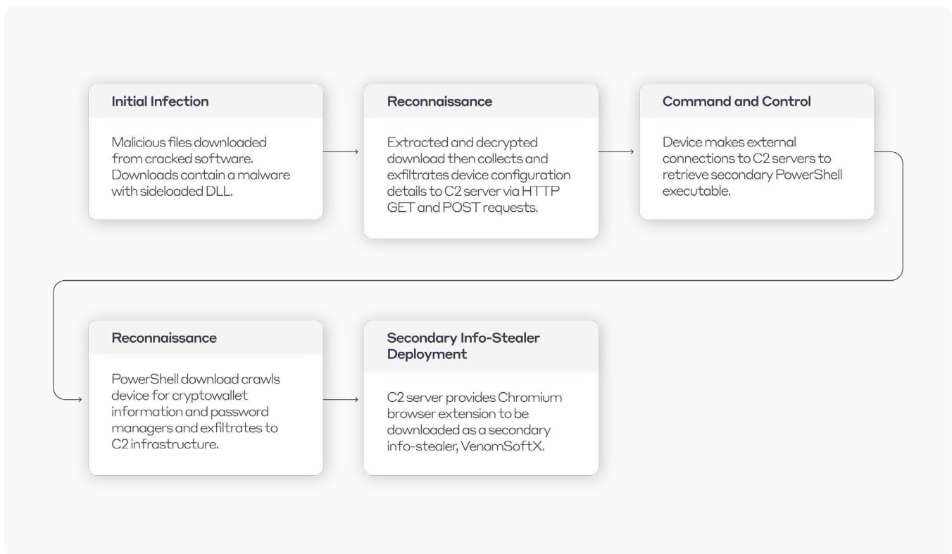
Figure 2: A typical attack progression of ViperSoftX malware observed by Darktrace.
